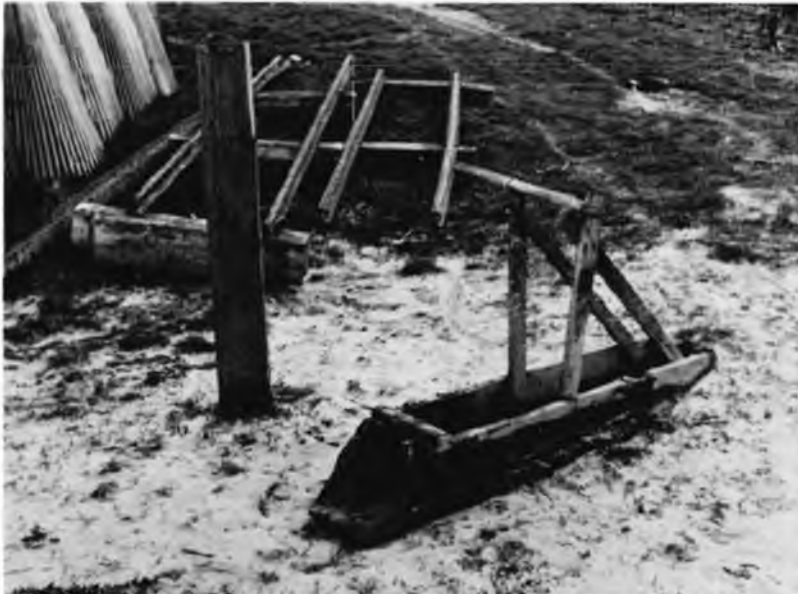
Fig. 23. Mud sled used on the western coast of the North Sea. By the courtesy of Dr. von Brandt.
